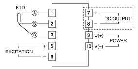
Note: The section enclosed by broken line is only with DC output option.
